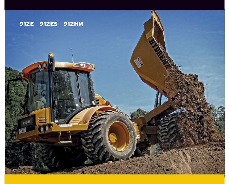
A unique combination of articulated center pivot, wide wheels and high ground clearance. For high mobility and low ground pressure.
